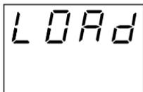
This indicates that the loading procedure has been initiated. After about 3 seconds the loading procedure is complete and the instrument reverts to the “normal display mode.” The following is a list of the default operating parameters loaded during the procedure:
