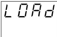
This indicates that the loading procedure has been initiated. After about 3 seconds the loading procedure is complete and the instrument reverts to the “CO<sub>N</sub>F” display. The following table is a list of the default configuration parameters loaded during the procedure:
