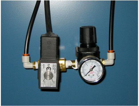
Connect Air line to right side of Regulator. Air should be clean and dry.
