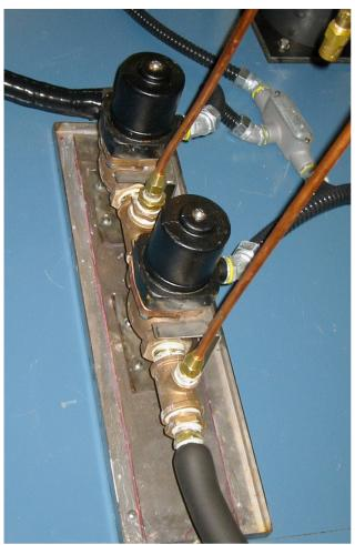
LN2 should be connected to Input of Regulator @ 75 PSI Max.
