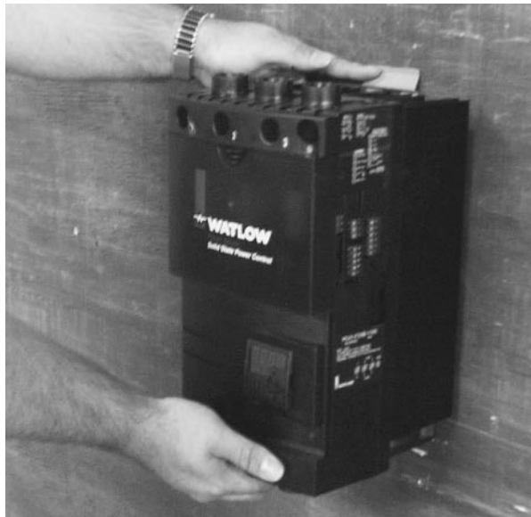
Figure 2.4 — Removing the controller.
