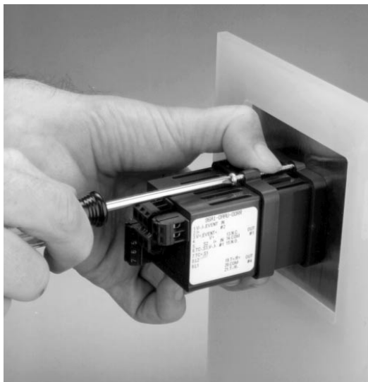
Figure 2.2a - Installing the controller.
